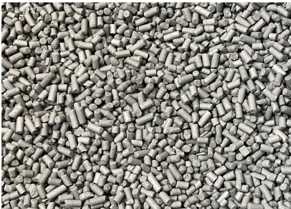
Photo: Typical Activated Carbon Media Granules of Diameter 4mm with length varying from 6 to 10mm.
