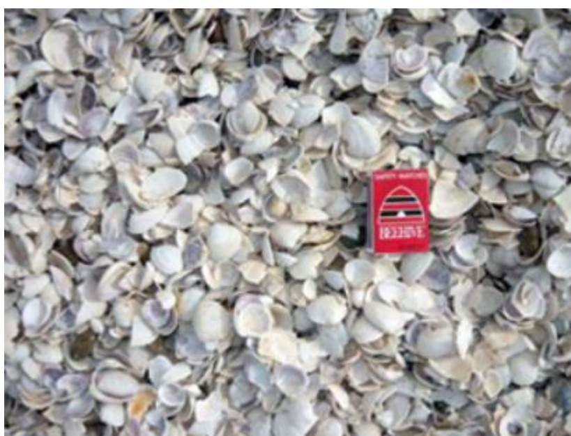
Photo: Shell size “13 Plus” (ie. \geq 13 mm)
