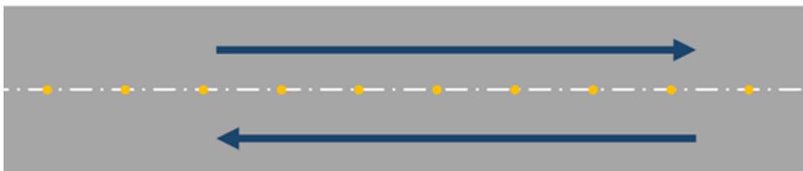
Figure 5: Delineator position – centre (separating lanes from each other)
