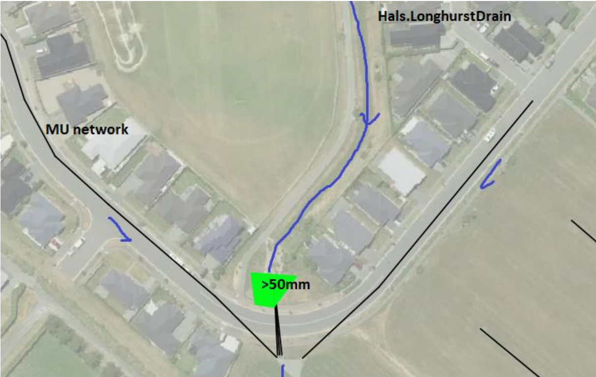
Figure 3-1: MIKE 21 oscillations at downstream end of Hals.LonghurstDrain
