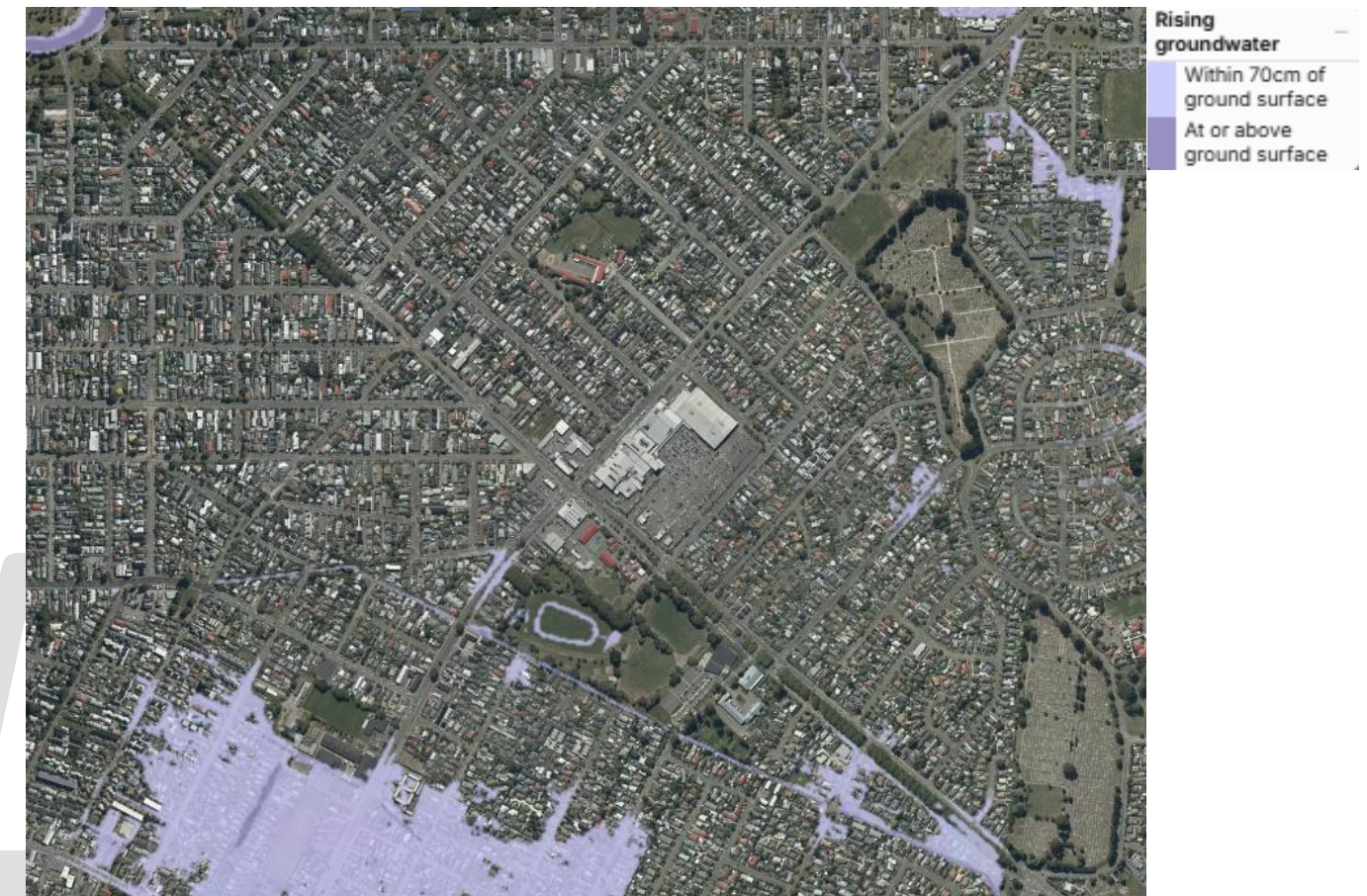
Figure 24: Rising groundwater with around 40 centimetres of sea-level rise, about 30 to 50 years from now.
