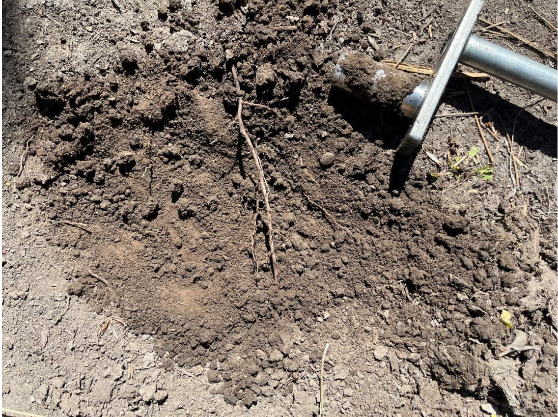
Photograph 7: Soil sample location BL_SS1_0.0 in the basin at Beckenham Library showing dry silty soil with some sand from 0 to 50 mm bgl.
